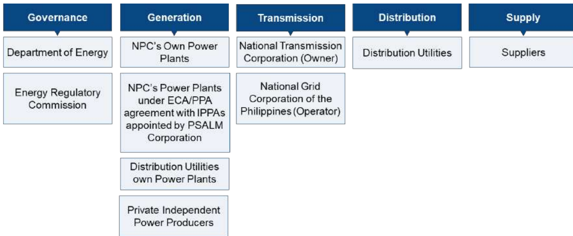
Figure 2-1: Electricity Industry Structure, the Philippines
